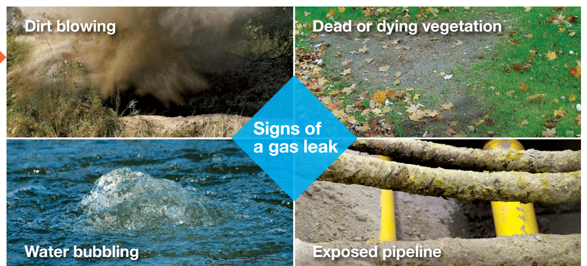
Leaking natural gas may throw dirt up into the air, kill grass or plants, or make bubbles in water. Gas pipelines exposed by fires or floods may be a source of leaks.
