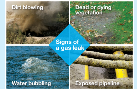
Leaking natural gas may throw dirt up into the air, kill grass or plants, or make bubbles in water. Gas pipelines exposed by fires or floods may be a source of leaks.
