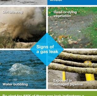
Be alert for ANY of these gas leak indicators: a distinctive, sulfur-like odor; continuous bubbling in water; a hissing, whistling or roaring sound; dirt blowing into the air from a hole in the ground; dead or dying vegetation (in an otherwise moist area) over or near a pipeline; an exposed pipeline after a fire or flood; or a damaged connection to a gas appliance. Know the procedures for gas leaks and fires.
