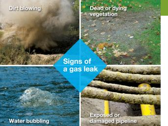
Be alert for ANY of these gas leak indicators: a distinctive, sulfur-like odor; continuous bubbling in water; a hissing, whistling or roaring sound; dirt blowing into the air from a hole in the ground; dead or dying vegetation (in an otherwise moist area) over or near a pipeline; an exposed pipeline after a fire or flood; or a damaged connection to a gas appliance.
