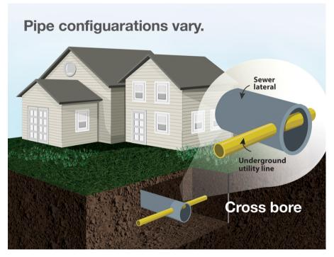
A natural gas line that is bored through a sewer lateral will impede the flow of sewage and eventually lead to a blockage. If you attempt to remove the blockage with mechanical equipment, you risk not only damaging the pipeline, but also injury to personnel as well as property damage. Gas may leak and travel into nearby sewer lines and buildings, causing a fire and explosion risk.
