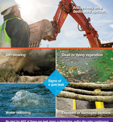
Be alert for ANY of these gas leak signs: a distinctive, sulfur-like odor; continuous bubbling in water; a hissing, whistling or roaring sound; dirt blowing into the air from a hole in the ground; dead or dying vegetation (in an otherwise moist area) over or near a pipeline; an exposed pipeline after a fire, flood or other disaster; or a damaged connection to a gas appliance.
