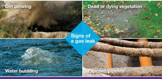
Leaking natural gas may throw dirt up into the air, kill grass or plants, or make bubbles in water. Gas pipelines exposed by fires or floods may be a source of leaks. These pipelines may be
