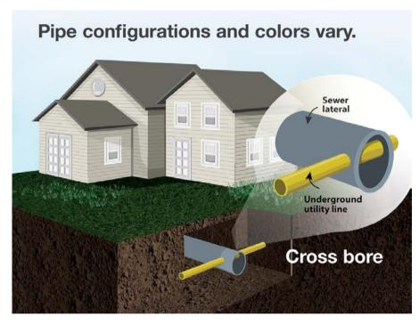
A natural gas line that is bored through a sewer lateral will impede the flow of sewage and eventually lead to a blockage. If you attempt to remove the blockage with mechanical equipment, you risk not only damage to the pipeline but also injury to personnel and damage to property. Gas may leak and travel into nearby sewer lines and buildings, causing a fire and explosion risk.
