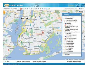
NPMS is a web-based mapping application, featuring data related to hazardous liquid and natural gas transmission pipelines, liquefied natural gas plants, and break-out tanks (a type of storage tank). NPMS does not include distribution lines or gathering pipelines that transport gas from wells to processing plants.
