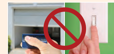
Danger! A spark from a garage door opener, light switch, cell phone or other electrical device can ignite leaking gas.
