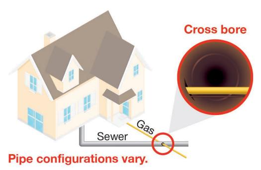
A cross bore in a sewer pipe will impede the flow of sewage and, eventually, lead to a blockage. Attempting to remove the blockage with mechanical equipment risks damaging a live utility line.
