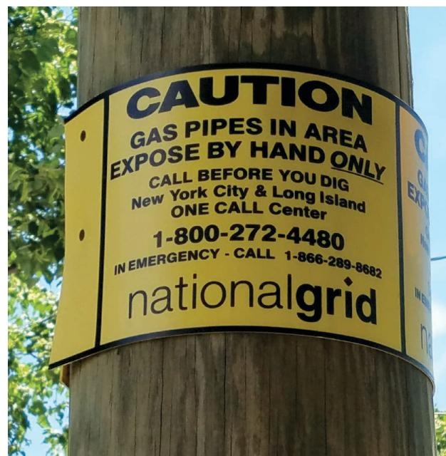
Natural gas pipeline markers are generally yellow and black. They're placed near pipelines but not necessarily directly on top of them.
