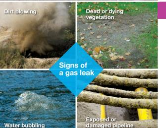
Be alert for ANY of these gas leak indicators: a distinctive, sulfur-like odor; continuous bubbling in water; a hissing, whistling or roaring sound; dirt blowing into the air from a hole in the ground; dead or dying vegetation (in an otherwise moist area) over or near a pipeline; an exposed pipeline after a fire or flood; or a damaged connection to a gas appliance.
