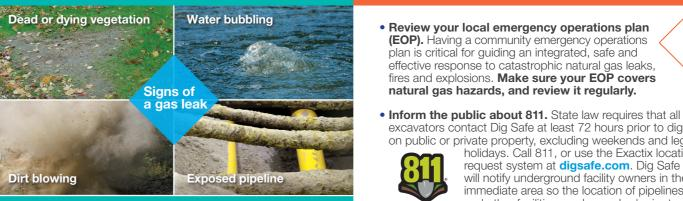
Leaking natural gas may throw dirt up into the air, kill grass or plants, or make bubbles in water. A damaged connection to a gas appliance and/ or pipelines exposed by fires or floods may be sources of leaks.
