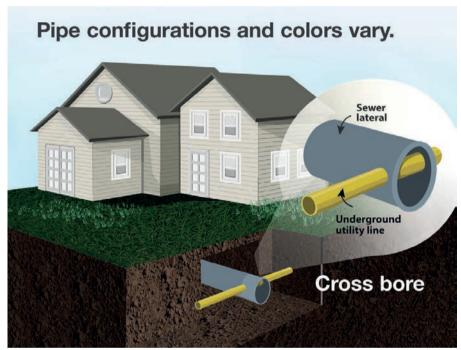
A natural gas line that is bored through a sewer lateral will impede the flow of sewage and eventually lead to a blockage. If you attempt to remove the blockage with mechanical equipment, you risk not only damage to the pipeline but also injury to personnel and damage to property. Gas may leak and travel into nearby sewer lines and buildings, causing a fire and explosion risk.
