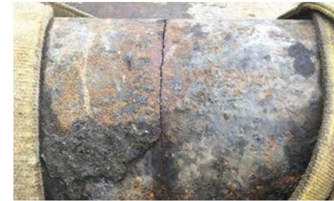
Cast iron gas mains are brittle and can break, endangering life and property when natural gas leaks.
