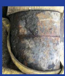
Cast iron gas mains are supported by the soil around them. **They can be damaged when the earth near them is moved in any way.** When possible, work with National Grid to plan your excavation to avoid damage to cast iron mains.
