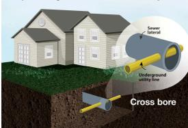
A natural gas line that is bored through a sewer lateral will impede the flow of sewage and eventually lead to a blockage. If you attempt to remove the blockage with mechanical equipment you risk not only damage to the pipeline but also injury to personnel and damage to property. Gas may leak and travel into nearby sewer lines and buildings, causing a fire and explosion risk.
