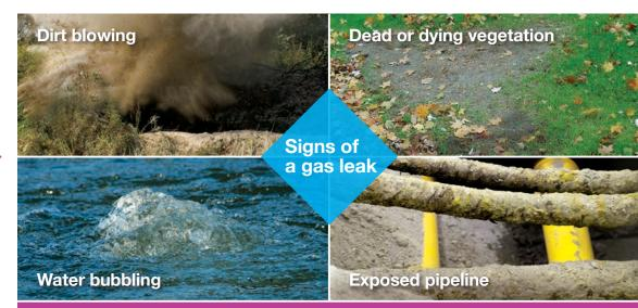
Leaking natural gas may throw dirt up into the air, kill grass or plants, or make bubbles in water Gas pipelines exposed by fires or floods may be a source of leaks.
