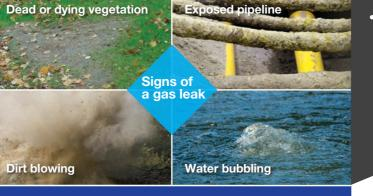
Leaking natural gas may kill grass or plants, make bubbles in water or throw dirt up into the air. Pipelines exposed by fires or floods may be sources of leaks, as may a damaged connection to a gas appliance.
